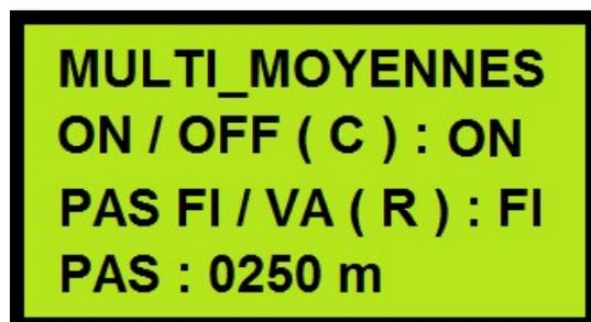
**R:** R key allows to choose between a fixed or a variable STEP ("PAS" in french).
